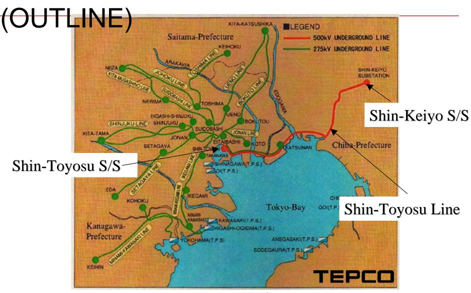
Aluminum covered XLPE (CAZVI) 2,500 mm<sup>2</sup>, 39.5 km, 2 circuits, 900MW/cct
